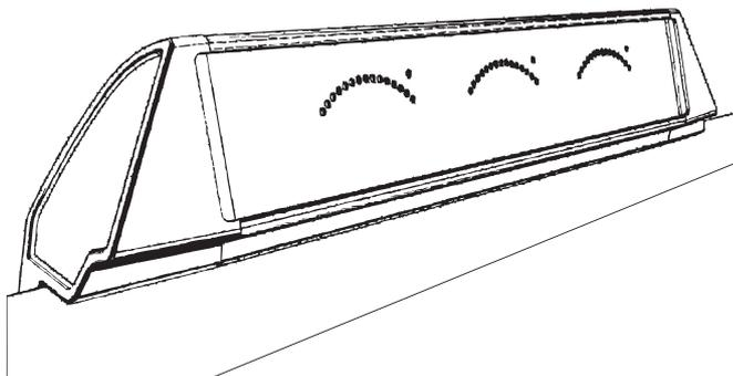
When the claws are located in the holes tip the meter bridge back to its upright position. Ensure that the ribbon cable hasn't been trapped. See Fig.3.
