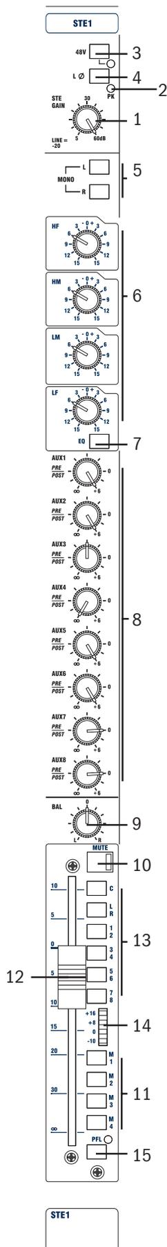
STE GAIN (1) adjusts the sensitivity of both pairs of Mic (XLRs) or Line (1/4" jacks) inputs. Both pairs are electronically balanced, and are located on the rear connector panel.
