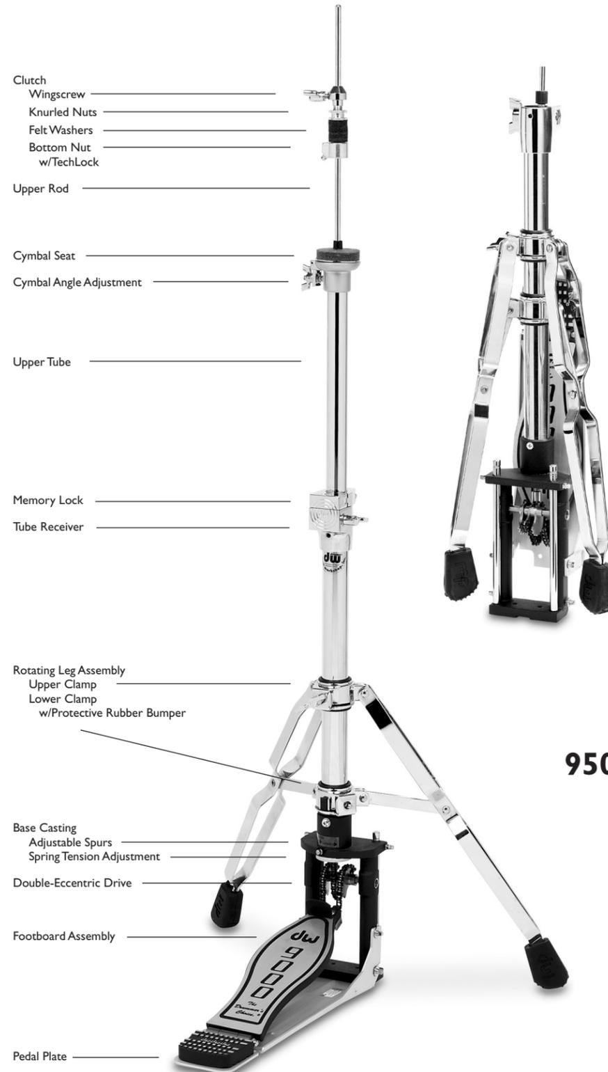
quality. To adjust the angle, turn the wingscrew while playing the pedal to achieve the desired sound. Once the optimal position is achieved, tighten the inside nut against the wingscrew to lock the angle/position
